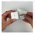
Step 3: Remove the battery from the controller.
